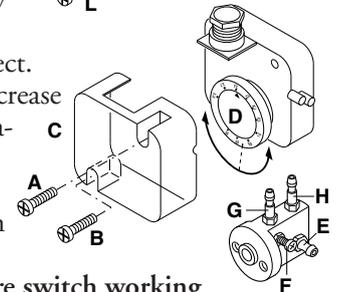
**Note:** The pressure measured at pressure port E must be within the limits of the pressure switch working range. If not, loose the locking nut of screw F and gradually turn the same: clockwise to reduce the pressure; counterclockwise to increase. At the end tighten the locking nut.
